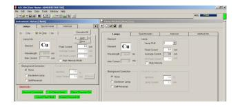
The TRACE software is designed to give users compete control of all parameters required to achieve optimal instrument performance. The software's periodic-table-driven interface allows users to easily retrieve and modify the pre-developed method database.
