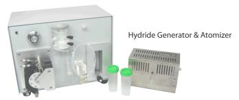
This system comes complete with an advanced gas-liquid separator which allows users to add a drying agent. By removing moisture, pressure fluctuations are minimized, thus enhancing the precision of measurements. Three mixing levels in the reaction/mixing manifold enable the convenient online addition of reagents required for acidity adjustments, pre-reduction/oxidation or masking of interferences.
