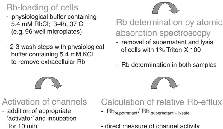
**Figure 8.4** Schematic representation of the experimental workflow for the non-radioactive rubidium efflux assay.
