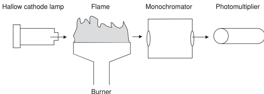
**Figure 8.3** Schematic diagram of an atomic absorption spectrometer (AAS). Copyright Wiley-VCH Verlag GmbH & Co. KGaA. Reproduced with permission.
