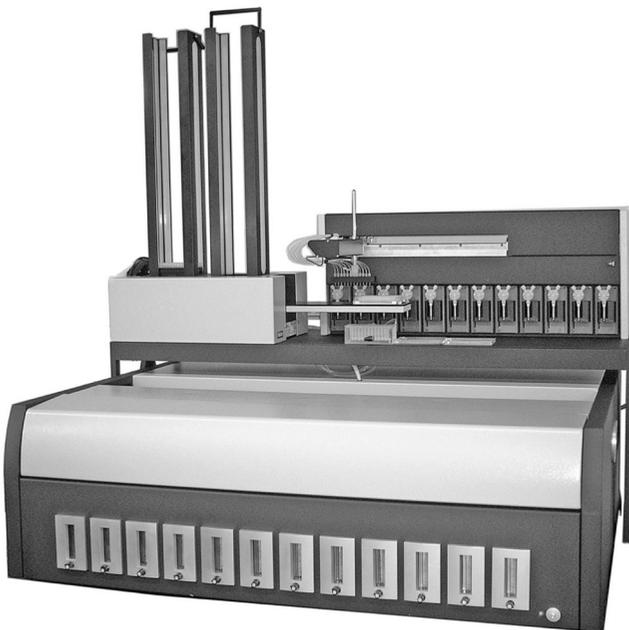
**Figure 8.5** Photograph of the Ion Channel Reader 12000 for parallel rubidium efflux AAS measurements of ion channels.
