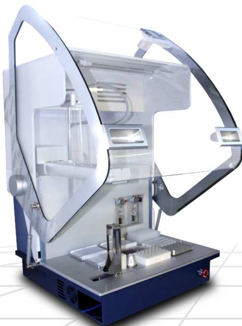
VERSA 110 NAP / PCR Setup Workstation with HEPA / UV / Fluorescent light enclosure
