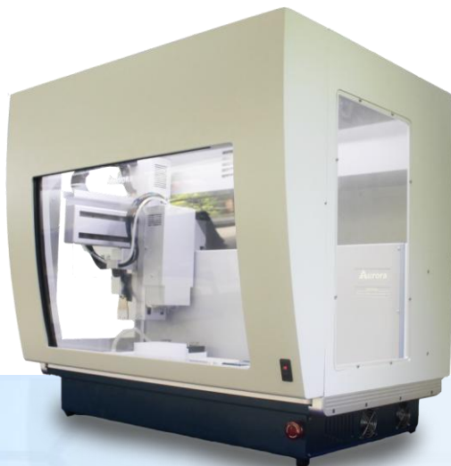
VERSA Gene 1100 Liquid Handling Workstation
