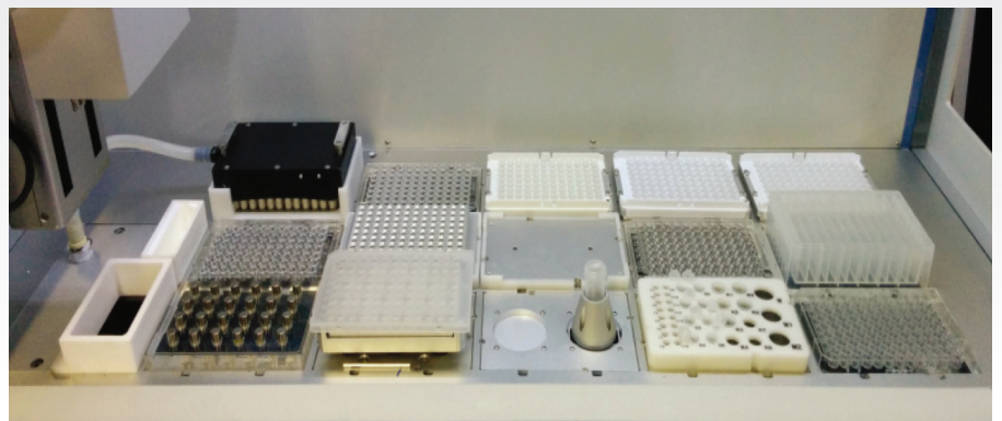
Figure 3: The deck layout of VERSA 1100 Workstation
