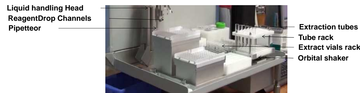
Figure 2: Deck layout of the VERSA Workstation for Copper stripping and extraction.
